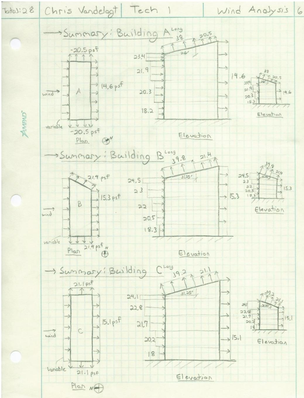
Figure 7: Summary of wind pressures normal to long dimension
