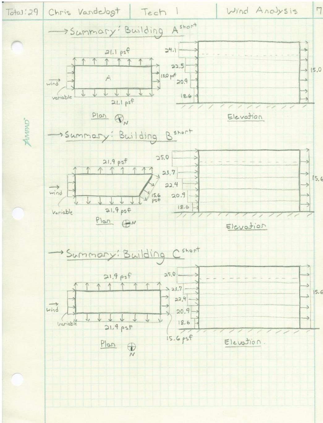
Figure 8: Summary of wind pressures normal to short dimension
