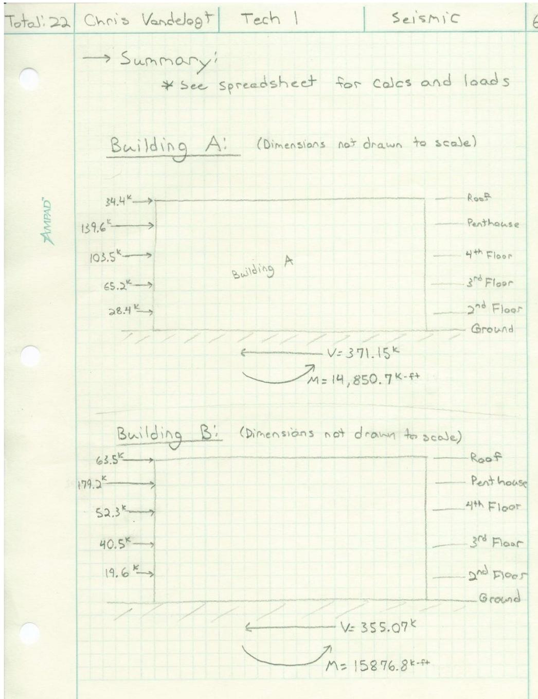
Figure 10: Summary of seismic loading
