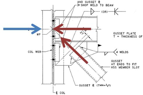
Figure 17: Lateral load path through a HSS cross braced connection. Courtesy of RIT.
