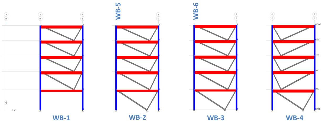
Figure 15: Elevations of braced frames in the Y-Direction modeled in ETABS
