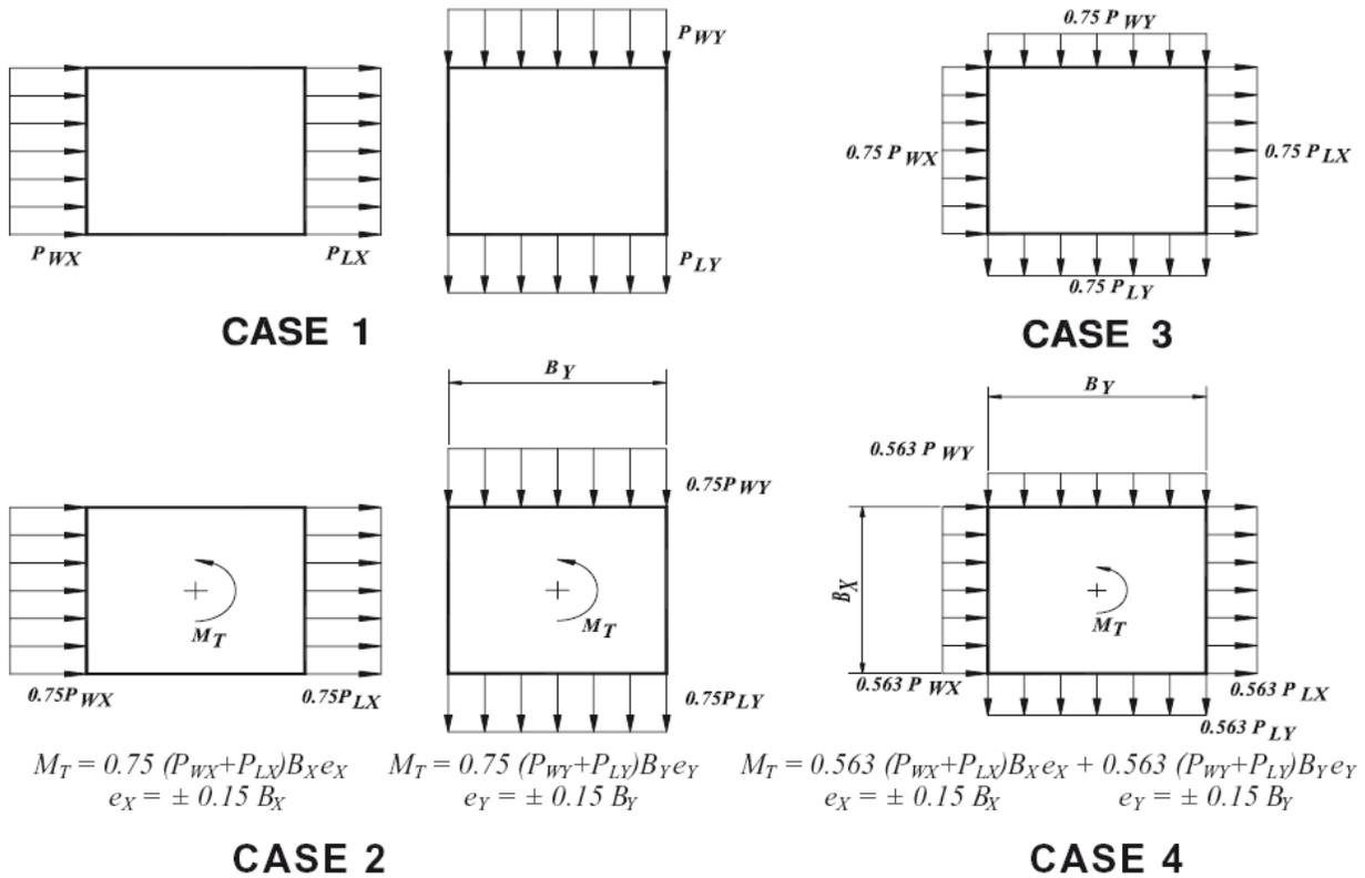
Figure 16: Wind load cases used in ETABS. Courtesy of ASCE 7-10 Figure 27.4-8.
