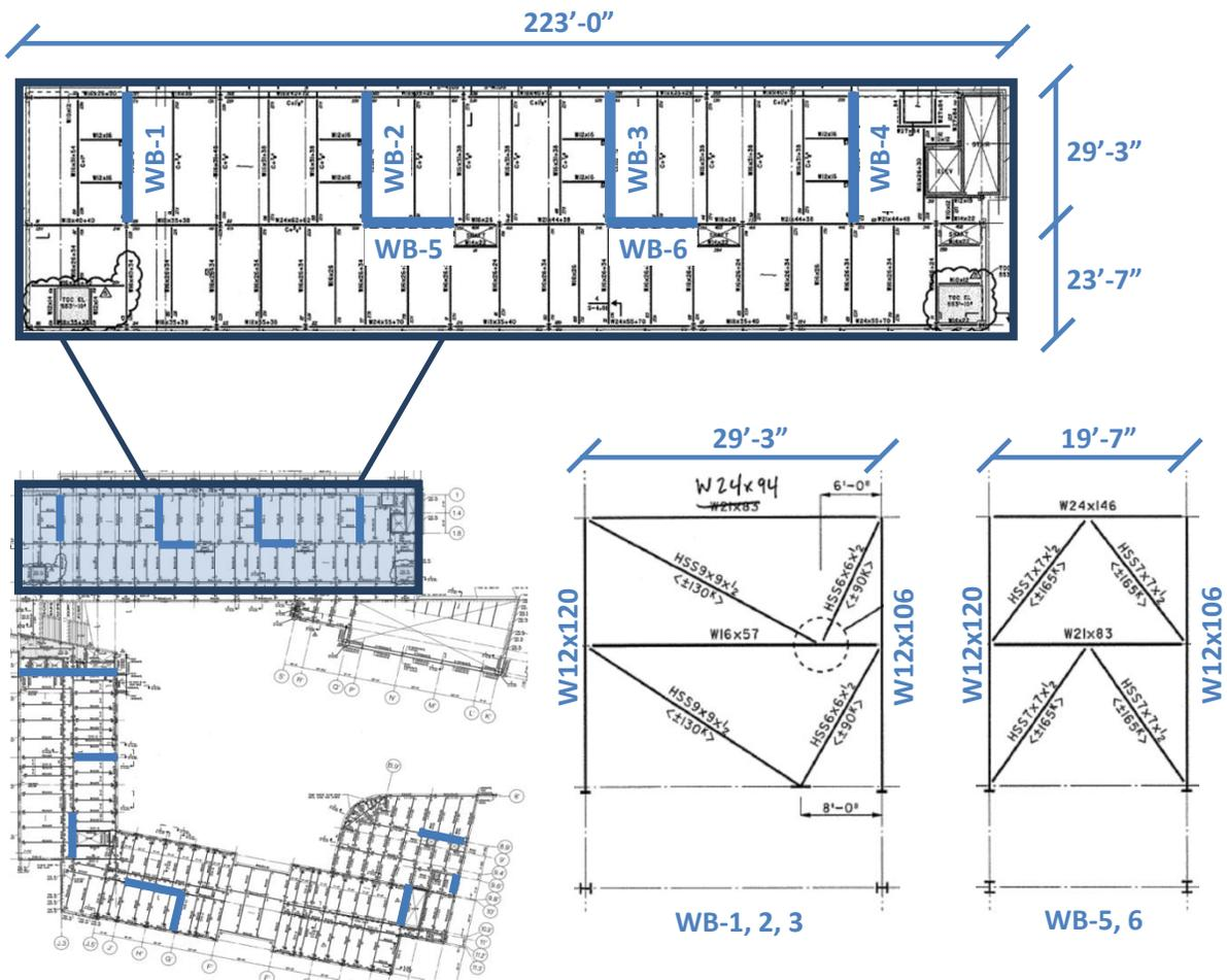
Figure 11: Typical bracing details and placement of bracing on 2nd Floor of the north leg. Courtesy of RIT. Drawings not to scale.
