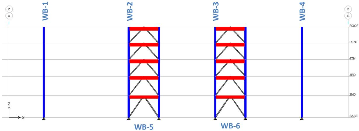
Figure 14: Elevation of braced frames in the X-Direction modeled in ETABS
